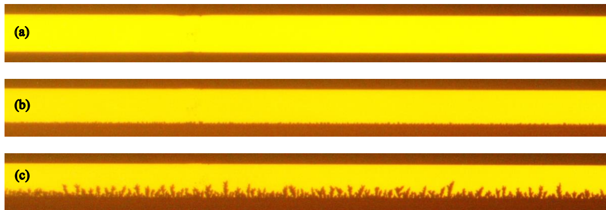
Figure 1: A typical electrodeposition experiment in which top electrode is anode (higher potential) while bottom electrode is cathode (lower potential). Images were taken at different times. (a) Initial flat surface. (b) Cellular formation starts which can be seen as roughening of cathode. (c) Cells continue to grow and form dendrites. cf Ref [1]
